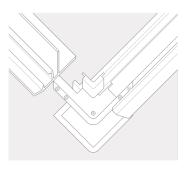
If required, secure corner pieces using screws provided.
