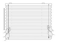
**To lower blind:** Move lift cord towards middle of the blind pulling down gently until cord lock releases.
