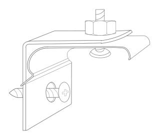
Feed the headrail into the brackets as shown and push headrail up at the rear until it clicks in place fully.
